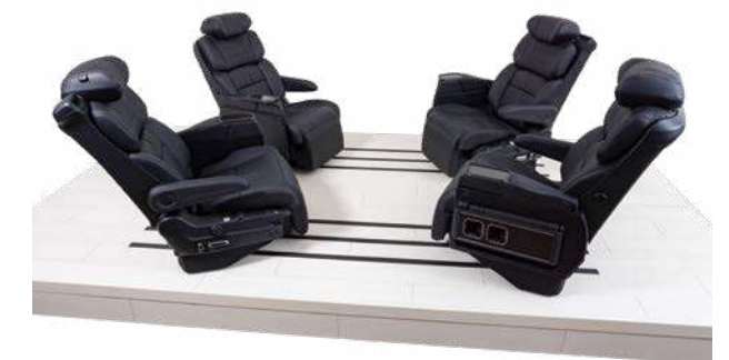
An extended slide rail that makes it possible to create large spaces, no matter where you sit with just a simple operation
